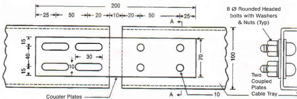
Coupler Plates (CTC) Typical for Lader type and perforated Type Trays
